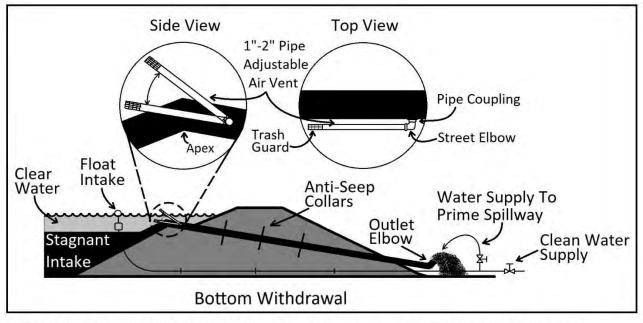
Figure 3. Cross-sectional view of a bottom-withdrawal spillway installation.
